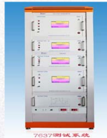
Vehicle interference simulator ISO7637 system
